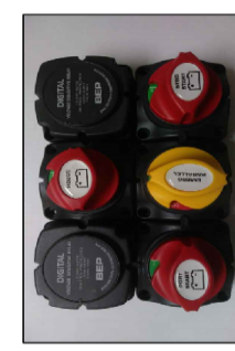
DETAIL-A BEP BATTERY DISTRIBUTION PANEL SEE DWG#285502 FOR OPERATION
